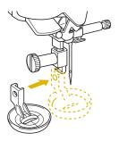
Tighten the screw with the included screwdriver.
