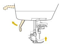
Push the black button on the presser foot holder and remove the presser foot.
