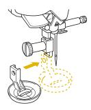
Tighten the screw with the included screwdriver.
