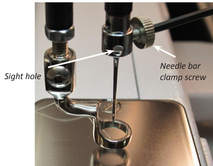
4. Remove the old needle by pulling it down. Discard the old needle in a safe way.
