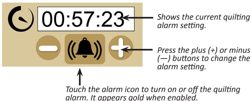
1. Specify the amount of time that will elapse before the alarm will go off. Fine tune the alarm setting by pressing the plus (+) or minus (-) buttons which changes the alarm setting by one minute at a time.
