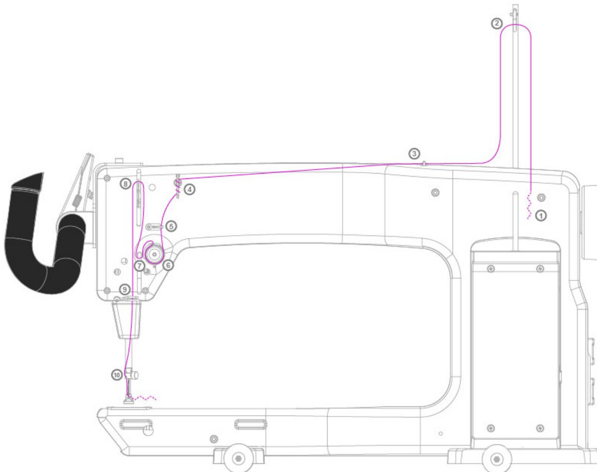
1. Place thread cone onto spool post ①, insert the thread through the thread-antennae eyelet ② from back to front, continuing to the thread guide ③.
