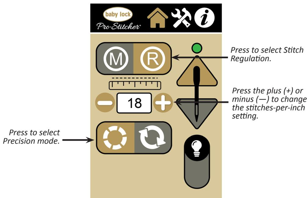
After you press the Start/Stop button on the handlebars, you must begin moving the machine for it to begin quilting according to the stitches-per-inch setting. When you begin moving the machine, stitching begins. When you stop moving the machine, stitching stops but just until you move it again.
