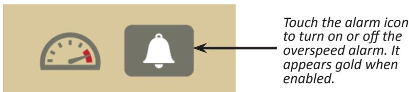
1. Touch the alarm button to turn it on or off. It is on when it appears gold with the sound-wave symbols. It is off when it appears gray.
