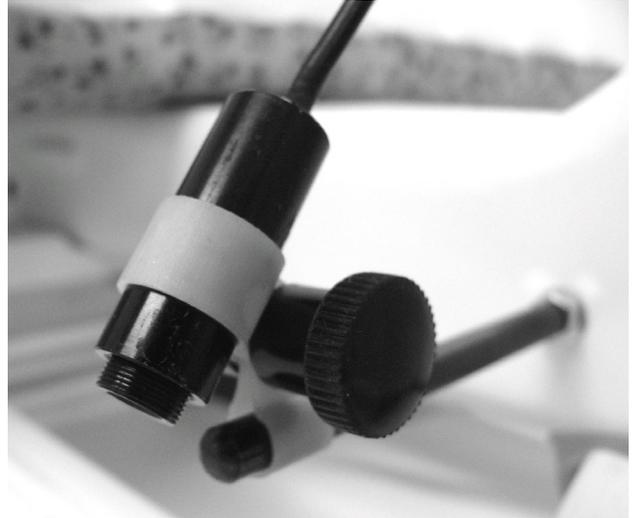
2. Insert the laser light stylus into the laser clamp.
