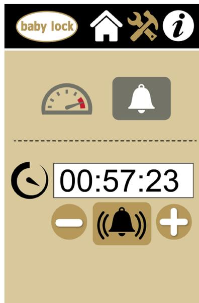
*The overspeed alarm alerts you if you are moving the machine faster than 100% of the motor capacity.*
