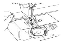
→ A loop of the bobbin thread comes out through the hole in the needle plate.
