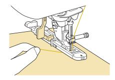
→ Once sewing is completed, the machine automatically sews reinforcement stitches, and then stops.
