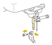
Set the adapter on the presser foot bar, aligning the flat side of the adapter opening with the flat side of the presser bar. Push it up as far as possible, and then tighten the screw securely with the screwdriver.
