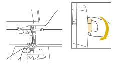
Gently pull the upper thread to bring the bobbin thread up through the needle plate.
