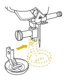
Tighten the screw with the included screwdriver.
