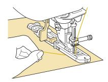
→ Once sewing is completed, the machine automatically sews reinforcement stitches, and then stops.
