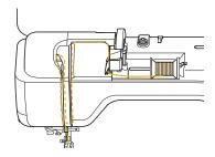
Pass the thread through the needle bar thread guides on the needle bar, then thread the needle on the left side manually.
