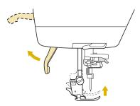
Push the black button on the presser foot holder and remove the presser foot.
