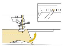
The pivot setting is useful when changing the sewing direction. When the machine is stopped at the corner of the fabric, the machine stops with the needle in the fabric and the presser foot is automatically raised so the fabric can easily be rotated ("Pivoting" on page S-15).
