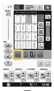
→ The key appears as , the quilting foot is raised to the necessary height, then the feed dogs are lowered for free motion sewing.
