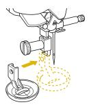
Tighten the screw with the included screwdriver.
