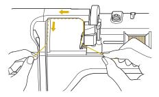
Guide the thread down, up, then down through the groove, as shown in the illustration.
