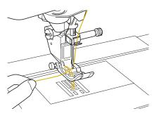
Pull up the bobbin thread, pass it under the presser foot and pull it about 100 mm (approx. 4 inches) toward the back of the machine, making it even with the upper thread.
