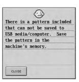
This message is displayed when you try to save a copyright protected pattern to USB media/ Computer. According to copyright laws, patterns that are illegal to reproduce or edit cannot be saved to USB media/Computer. If this message displays, save the pattern in the machine's memory.
