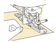
→ A buttonhole starts to sew from the front of the presser foot to the back.
