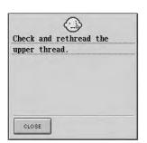
This message is displayed when the upper thread is broken or not threaded correctly, and the "Start/ Stop" button or the "Reverse/ Reinforcement Stitch" button is pressed.
