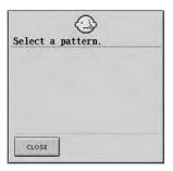
This message is displayed when the "Start/Stop" button, "Reverse/ Reinforcement Stitch" button is pressed while no pattern is selected.
