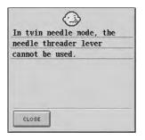
This message is displayed when you try to use the needle threader lever while twin needle sewing is set.
