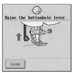
This message is displayed when a stitch other than a buttonhole stitch is selected and the "Start/Stop" button or the "Reverse/ Reinforcement Stitch" button is pressed while the buttonhole lever is lowered.
