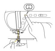
Gently pull the upper thread to pull up the bobbin thread.
