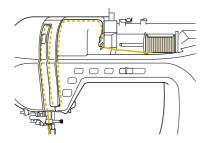
Pass the thread through the needle bar thread guide, and then thread the needle on the left side
