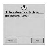
This message is displayed when NO. is pressed while the presser foot is raised.
