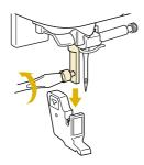
Set the operation lever of the walking foot so that the needle clamp screw is set between the fork, and position the walking foot on the presser foot bar.
