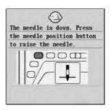
This message is displayed when the machine is turned on while the needle is lowered and the embroidery unit is attached.
