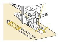
When sewing is finished, gently pull the gimp thread to remove any slack, and then use a handsewing needle with a large eye to pull the gimp thread to the wrong side of the fabric.
