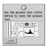
This message is displayed when the "Start/Stop" button, "Reverse/ Reinforcement Stitch" button, or the "Thread Cutter" button is pressed while the presser foot and the needle are raised.
