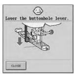
This message is displayed when a buttonhole stitch is selected and the "Start/Stop" button or the "Reverse/Reinforcement Stitch" button is pressed while the buttonhole lever is raised.
