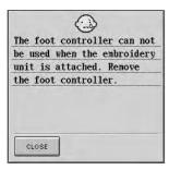
This message is displayed when the foot controller is pressed while the embroidery unit is attached.
