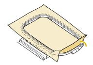
Gently stretch the fabric, and then securely tighten the frame adjustment screw so that the fabric remains stretched.
