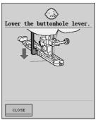
This message is displayed when the buttonhole lever is up, a buttonhole stitch is selected, and the "Start/ Stop" button or "Reverse/Reinforcement Stitch" button is pushed.
