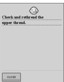
This message is displayed when the upper thread is broken or not threaded correctly, and the "Start/Stop" button or the "Reverse/ Reinforcement Stitch" button is pressed.
