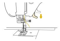
Holding the thread with both hands, pass the thread through both the upper and lower needle bar thread guides.
