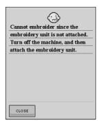
This message is displayed when the "Start/Stop" button is pushed and the machine is in embroidery mode, but the embroidery unit is not attached.
