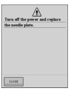
This message is displayed when you try to sew with a stitch other than a middle needle position stitch while the single-hole needle plate is installed. This message is displayed when the needle plate is removed with the machine on or when the machine is turned on in the embroidery or embroidery edit
