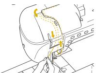
Do not pass the thread in the needle bar thread guides on the needle bar. Thread the needle on the right side.
