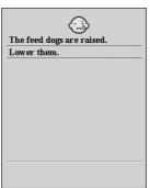
This message is displayed when the "Start/Stop" button is pushed without raising the feed dogs after the feed dogs are lowered or after the embroidery unit is attached.
