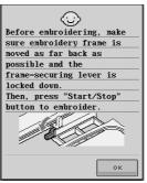
This confirmation message appears after the machine is turned on and the carriage of the embroidery unit has moved to its initial position.
