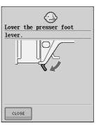
This message is displayed when the "Presser Foot Lifter" button is pushed while the presser foot lever is raised/the needle is lowered.
