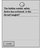
This message is displayed when the bobbin is being wound, and the motor locks because the thread is tangled, etc.
