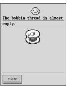
This message is displayed when the bobbin thread is running out.
