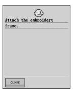
This message is displayed when the machine is ready to sew an embroidery pattern, and the "Start/Stop" button is pushed while the embroidery frame is not attached.
