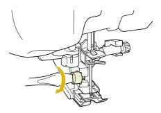
Place one hand on each side of the presser foot to hold the fabric secure while sewing.
