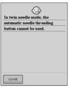
This message is displayed when the automatic needle threading button is pushed while twin needle sewing is set.
