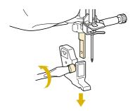
Set the operation lever of the walking foot so that the needle clamp screw is set between the fork, and position the walking foot on the presser foot bar.
