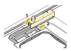
Insert a wound bobbin into the machine, then reattach the embroidery frame.
