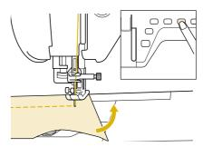
When edge stitching a short stitch length close to the edge of the fabric, the presser foot may not cover enough fabric for proper feeding. Before you begin to sew, sew a basting thread at the corner point. When you change direction at the corner, start sewing as you pull the basting thread toward the back.
