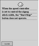
This message is displayed when the speed control lever is set to control the zigzag stitch width, and the "Start/ Stop" button is pushed. Use the foot controller to operate the machine.
