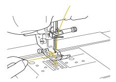
Pull up the bobbin thread, then pass it under the presser foot and pull it about 100 mm (approx. 3-4 inches) toward the back of the machine, making it even with the upper thread.
