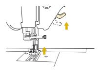
Pivot the spool pin so that it angles upward. Set the thread spool on the spool pin so that the thread unwinds from the front of the spool.
