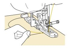
→ When sewing is completed, the machine will sew reinforcement stitches and stop automatically.
