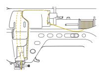
Pass the thread through the needle bar thread guides on the needle bar, then thread the needle on the left side.
