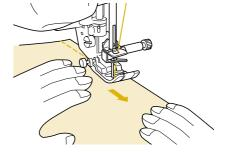
End the basting with reinforcement stitches.
