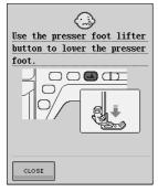
This message is displayed when a button, such as the "Start/Stop" button, is pushed while the presser foot is raised.
