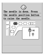
This message is displayed when the embroidery unit is attached and the power is turned on with the needle in the down position.
