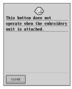
This message is displayed when the "Reverse/Reinforcement Stitch" button is pushed while the embroidery unit is attached.
