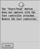
This message is displayed when the "Start/Stop" button is pushed to sew Utility stitches or Character/Decorative stitches while the foot controller is connected. (This message does not appear when embroidering.)
