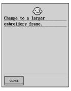
This message is displayed when the machine is in embroidery mode and the small frame is attached, and the selected pattern does not fit in the small frame
