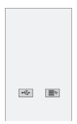
Insert the USB media into the USB port connector on the machine, making sure the media only contains the upgrade file.
