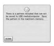
This message is displayed when you try to save a copyright protected pattern to USB media/Computer. According to copyright laws, patterns that are illegal to reproduce or edit cannot be saved to USB media or computer. If this message displays, save the pattern in the machine's memory.
