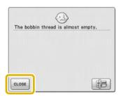
Note If "Upper and Bobbin Thread Sensor" in the General settings screen of the machine setting mode is set to "OFF", the message shown above does not appear.
