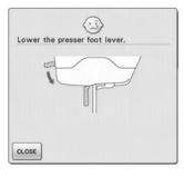
This message is displayed when the "Presser Foot Lifter" button is pushed while the presser foot lever is raised/ the needle is lowered.
