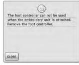
This message is displayed when the foot controller is pressed while the embroidery unit is attached and machine is set up for embroidering.
