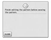
This message is displayed when the "Start/ Stop" button is pushed while the machine is in embroidery edit mode and a pattern is being edited.
