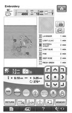
The fabric hooped in the embroidery frame can be displayed on the LCD so that the embroidery position can be easily aligned.
