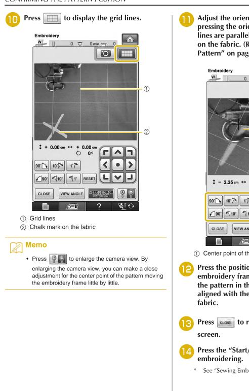
Adjust the orientation of the pattern by pressing the orientation keys until the grid lines are parallel with the chalk mark drawn on the fabric. (Refer to "Rotating the Pattern" on page 242.)
