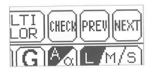
After a lot of text has been typed in, it may not be possible to view some of it on the screen. Press the **CHECK** key for the entire text to scroll across the screen.
