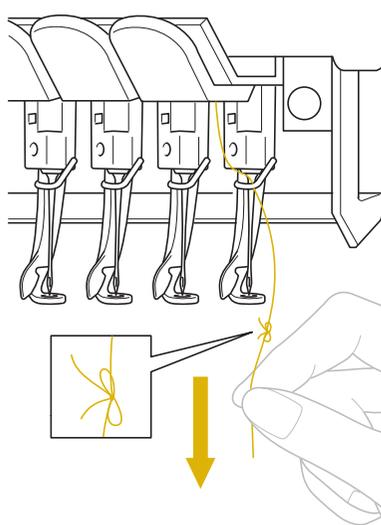
Continue pulling the thread until the knot is above the needle. Cut the knot.
