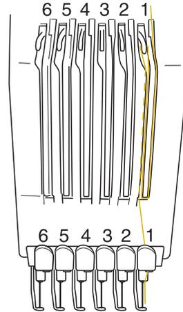
**3** Pass the thread through the hole in the number 1 upper thread guide. Pass the thread toward you from the inside of the thread guide.
