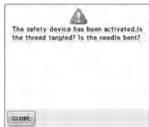
The motor has locked up due to tangled thread or for other reasons related to thread delivery.
