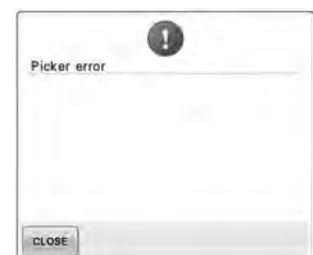
The thread picker did not operate correctly. Remove the thread entangled on the thread picker.
