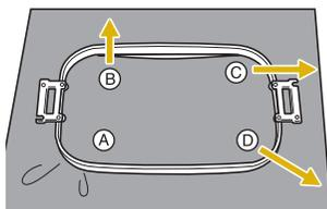
First, align the inner and outer frames at the corner with the screw (A). Then, while lightly pulling the fabric in the direction indicated by arrow (B) so that the fabric is taut, insert the inner frame at corner (B). In the same way, lightly pull the fabric in the direction indicated by arrow (C) and insert corner (C),
