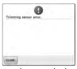
Dust may have accumulated within the moving cutter. Clean the moving cutter. (Refer to page 278.)
