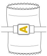
**Example:** When embroidering a T-shirt Rotate the pattern 180 degrees. Pass the machine bed through from the waist of the T-shirt, not from the neck, and attach the embroidery frame to the machine. This will prevent the neck of the shirt from being stretched when the embroidery frame is moving.
