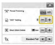
A value between 1 and 8 can be specified. For example, if 3 is specified, sequential 3 jump codes will be converted to the trim code. But sequential 2 jump codes will not be converted to the trim code, it will be sewed as the feed (jump) stitch.
