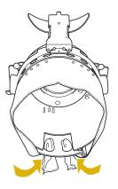
6 Lift out the sweat guard on the inside of the cap, and then place the cap over the cap frame.
