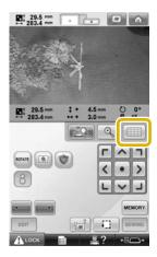
Touch the positioning keys to move the embroidery frame until the thread mark on the fabric is aligned on the starting point in the camera view window.
