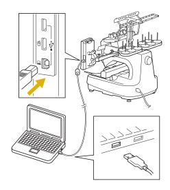
If the machine is positioned at a distance that prevents the USB cable from reaching the computer, embroidery patterns can be transferred from the computer by temporarily saving them on USB media, which is then connected to the machine. (Refer to "USB media" on page 172.)
