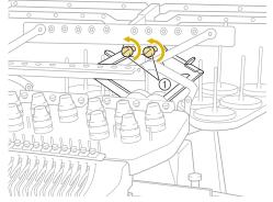
① Turn the screw counterclockwise three or four times to loosen it.
