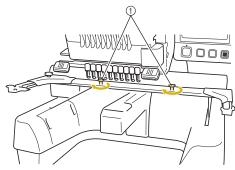
(1) Use the thumb screws included with the machine (thumb screws removed in step 1) on page 256).
