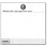
The needle bar case has stopped at The needle bar case motor has an incorrect position.
