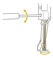
With the flat side of the needle toward the back of the machine, insert the needle all the way up until it touches the needle bar stopper.
