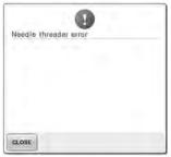
The automatic needle-threading mechanism did not operate correctly.
