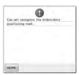
Machine failed to recognize the embroidery positioning mark. Confirm that the embroidery positioning mark is in the selected area. If problem persists, reposition the mark.
