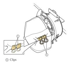
While pulling the lever toward you that is located behind the handle on the right side of the mounting jig, rotate the cap frame to the right.
