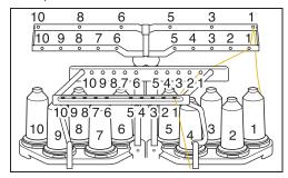
Pass the thread of a specified color through the holes on the thread guide, making sure that you have the thread color matched to the coordinating needle bar.
