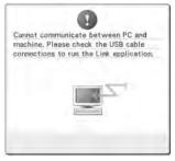
Machine cannot receive any data from the PC in the Link mode. Turn off the machine, and check the USB connection. After connect the USB cord securely, turn on the machine again. (Refer to page 174)
