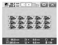
• When changing the direction in which the pattern will be repeated, all of the patterns in the red frame will automatically be grouped as one repeating unit. See the following section on how to repeat one element of a repeated pattern.
