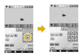
The pattern can also be moved by dragging it. If a USB mouse is connected, move the mouse to position the pointer on the desired pattern, and then while holding in the left mouse button, drag the pattern. The pattern can also be dragged by selecting it directly in the screen with your finger or the touch pen.
