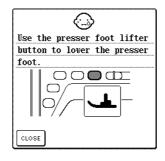
This message is displayed when the "Start/Stop" button, "Reverse/ Reinforcement Stitch" button, or the "Thread Cutter" button is pressed while the presser foot is raised.
