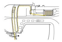
Pass the thread through the needle bar thread guide, and then thread the needle on the left side.
