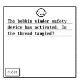
This message is displayed when the bobbin is being wound, and the motor locks because the thread is tangled, etc.
