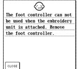
This message is displayed when the foot controller is pressed while the embroidery unit is attached.
