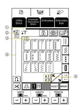
① Shows whether the machine is set for a single needle or twin needle, and the needle position when the machine is stopped. The desired needle position can be set (see page 20).
