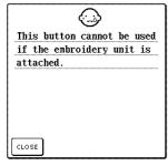
This message is displayed when the "Reverse/Reinforcement Stitch" button is pressed while the embroidery unit is attached.
