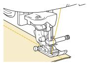
Press the "Thread Cutter" button to trim the threads.
