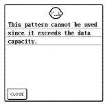
This message is displayed when you try to retrieve a pattern saved with the number of stitches or the number of colors exceeding the specified limits.
