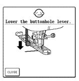
This message is displayed when a buttonhole stitch is selected and the "Start/Stop" button or the "Reverse/Reinforcement Stitch" button is pressed while the buttonhole lever is raised.
