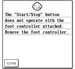
This message is displayed when the "Start/Stop" button is pressed while the foot controller is connected.
