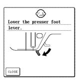
This message is displayed when the "Start/Stop"button, "Reverse/ Reinforcement Stitch" button, "Thread Cutter" button, or "Presser Foot Lifter" button is pressed while the presser foot lever is raised/the needle is lowered.
