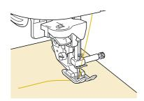
Press the "Reverse/Reinforcement Stitch" button to sew reinforcement stitches, and then press the "Start/Stop" button to start sewing.
