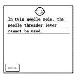
This message is displayed when you try to use the needle threader lever while twin needle sewing is set.
