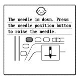
This message is displayed when the machine is turned on while the needle is lowered and the embroidery unit is attached.
