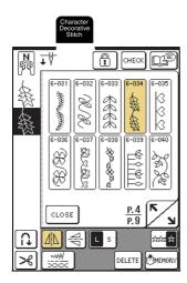
$\rightarrow$  The second pattern is flipped on a vertical axis.
