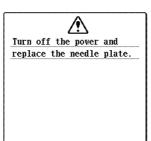
This message is displayed when you try to sew with a stitch other than a middle needle position stitch while the single-hole needle plate is installed.
