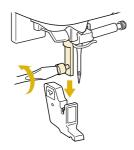
Set the operation lever of the walking foot so that the needle clamp screw is set between the fork, and position the walking foot on the presser foot bar.
