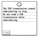
If data is being written to or deleted from "Removable Disk" on the connected computer during sewing, the machine stops and this message is displayed.
