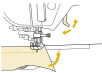
The pivot setting is useful when changing the sewing direction. When the machine is stopped at the corner of the fabric, the machine stops with the needle in the fabric and the presser foot is automatically raised so the fabric can easily be rotated (see "Pivoting" on page 47).
