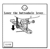
This message is displayed when a buttonhole stitch is selected and the "Start/Stop" button or the "Reverse/Reinforcement Stitch" button is pressed while the buttonhole lever is raised.
