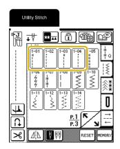
Set the stitch length to 4.0 mm (approx. 3/16 inch) and the thread tension to 2.0 (weaker tension).
