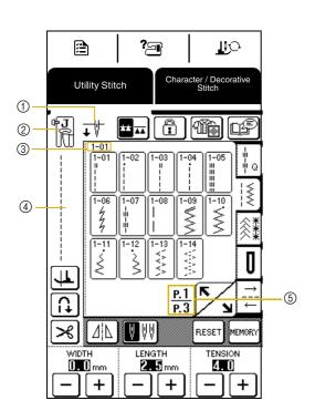
① Shows whether the machine is set for a single needle or twin needle, and the needle position when the machine is stopped. The desired needle position can be set (see page 22).
