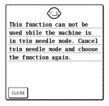
This message is displayed when the machine is set for twin needle sewing and a pattern that cannot be sewn with the twin needle is selected.
