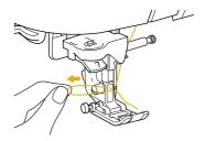
Pull out about 100 mm (approx. 3-4 inches) of the thread, and then pass it under the presser foot toward the rear of the machine.
