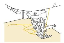
· After sewing is finished, trim any excess thread.
