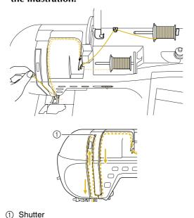
Without passing the thread through the needle bar thread guide, manually thread the needle on the right side.
