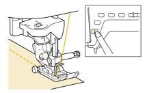
Press the "Thread Cutter" button to trim the threads.
