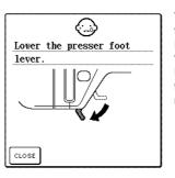
This message is displayed when the "Start/Stop" button, "Reverse/ Reinforcement Stitch" button. "Thread Cutter" button or "Presser Foot Lifter" button is pressed while the presser foot lever is raised/the needle is lowered.
