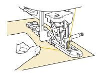
→ A buttonhole starts to sew from the front of the presser foot to the back.
