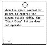
This message is displayed when the "Start/Stop" button is pressed while the sewing speed controller is set to control the zigzag stitch width.
