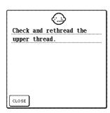
This message is displayed when the upper thread is broken or not threaded correctly, and the "Start/ Stop" button or the "Reverse/ Reinforcement Stitch" button is pressed.
