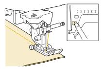
→ The machine stops with the needle in the fabric, and the presser foot is raised. Rotate the fabric, and then press the "Start/ Stop" button.
