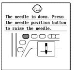
This message is displayed when the needle is in the down position and the needle threader is lowered.
