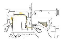
Guide the thread down, up, then down through the groove, as shown in the illustration.
