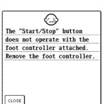
This message is displayed when the "Start/Stop" button is pressed while the foot controller is connected.
