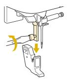
Position the free-motion echo quilting foot "E" on the left side of the presser bar with the holes in the quilting foot and presser bar aligned.
