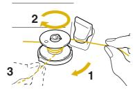
Pass the end of the thread through the guide slit in the bobbin winder seat, and then pull the thread to the right to cut it with the cutter.
