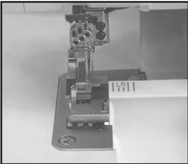
1. The chain stitch (C-3) combined with the 3 thread overlock is the most common 5-thread combination. The mark closest to the needles indicates 5/8 inch (16mm) from the cutting edge to the C-3 chain needle.
