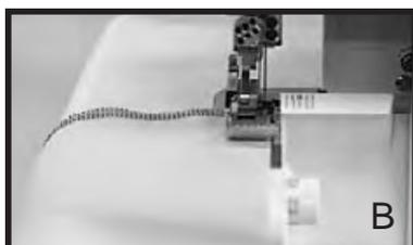
**Note:** A loose thread loop at the corner is caused by too much slack in the needle thread when clearing the stitch fingers. Try again, turning corners takes a little practice!
