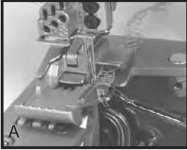
As you sew, you will discover that maneuvering the fabric is different from conventional sewing because the threads form around the stitch fingers (fig. A).
