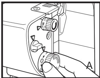
The stitch length / rolled hem adjusting dial is conveniently located just to the left of the front cover, near the base plate (fig. A). The dial shows two stitch-length ranges, each numbered from 1, for the shortest stitch, to 4 for the longest. As the dial indicates, one range is for standard sewing and one is for rolled edging or narrow seaming.
