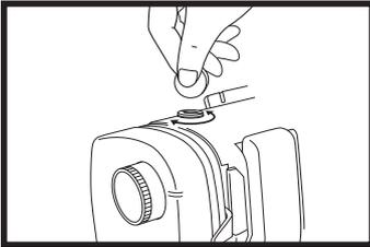
The presser foot pressure has been preset at the factory and rarely needs adjustment. You may find it necessary, however, to decrease the pressure for thick fabrics or increase pressure for thin fabrics to feed more smoothly under the foot. Use a coin to turn the screw on top of the machine. To increase pressure, turn the pressure adjusting screw clockwise. To decrease pressure, turn the screw counterclockwise.
