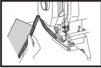
There is a thread cutter located on the left side of your evolve. At the end of a seam, sew off the fabric edge and continue sewing to create a 5-6 inch (12.5-15cm) thread chain. Bring the chain of thread up and from the back to front through the thread cutter.
