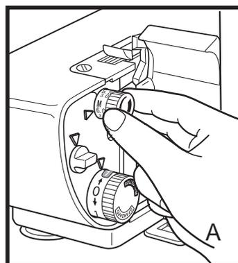
The stitch width adjusting dial is located above the stitch length dial (fig. A). The stitch width displays two sets of numbers, indicating two width ranges. For overlock stitches. The larger numbers at each end of the dial, 5.5 and 7.5mm, denote the stitch width when the 0-1 (left hand) needle is in use. The smaller numbers, 3.0 and 5.0mm, apply when only the 0-2 (right-hand) needle is in use for forming a 3-thread stitch. The "M" setting (3.5) is for the rolled edge.
