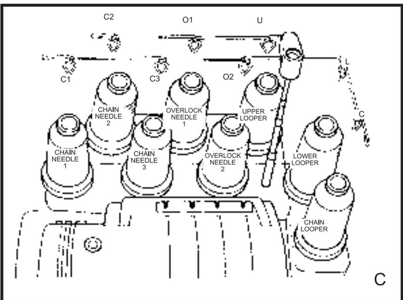
The spool pins, tension dials, thread guides, and threading ports are color coded for your convenience.
