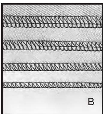
The stitch width is infinitely variable between either end of the range. Simply turn the dial aligning the desired setting with the indicator mark on the machine. Use a wider stitch on loosely woven fabrics. You may prefer a narrower stitch width on knits, tightly woven, or sheer fabrics (fig. B).
