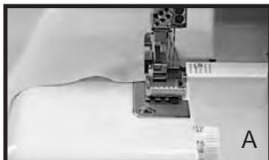
1. Stitch along one edge until you reach the corner. Take one stitch off the edge of the fabric (fig. A). (As you approach the edge, you may want to stop and manually turn the handwheel towards you.)
