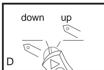
When you change from overlocking to chain/cover stitching, you should also change the upper looper positioning lever to the "DOWN" position before you close the sewing table door.
