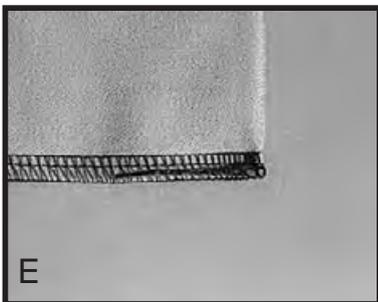
The serger stitch will not unravel readily, and in most cases serged seams are secured by an intersecting seam.
