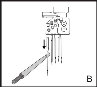
The overlock needles are on the back portion of the needle clamp and are identified by O-1 and O-2.
