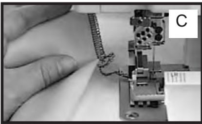
For "loops" (lower looper thread) to show on the right side, place fabric wrong sides together for sewing the seam. To produce the "ladder" (needle thread) on the outside, place the fabric right sides together (fig. B).
