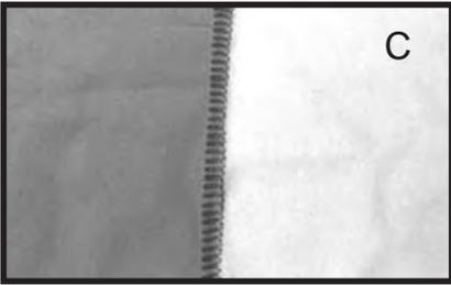
Set up the machine for 2-thread flatlock - wide but the needle threading path is different for this technique.
