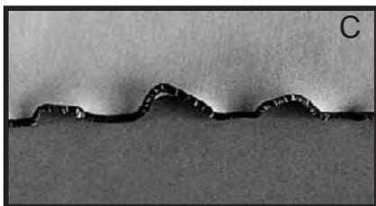
**Note:** To avoid the stitching from pulling away from the fabric, increase the width to a slightly larger number.
