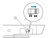
Drop feed lever (as seen from the rear of the machine)
