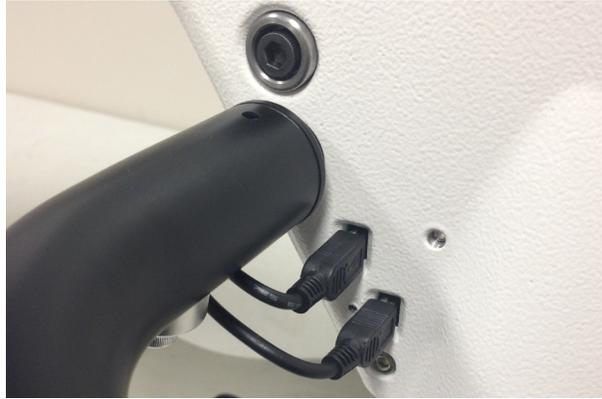
8. Each side of the handlebar can be individually adjusted forward or backward to a comfortable position for quilting. Loosen and tighten the handlebar lever bolt closest to the machine body. Fully hand-tighten the levers once in the desired position. Each side can also be adjusted in and out and rotated up or down as desired using the lever closest to the handle control switches.
