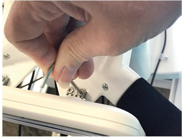
3. Plug the USB mini B cable with 90° end into the rear display and the straight end into the rear panel of the machine.
