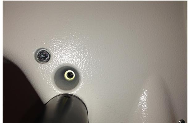
6. Place the wedge and M6x45 hex screw with washer into hole and start the screw into the threaded piece with your fingers. Once the screw is nicely started into the handle bar, firmly tighten the screw with the provided 5mm Allen wrench
