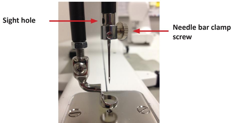
4. Remove the old needle by pulling it down. Discard the old needle in a safe way.
