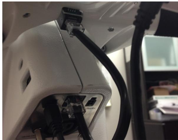
Connect the USB mini B connector to the back of the machine. You will need the other end for the display later. Note that this cable powers the display, the round power input to the display is not used.
