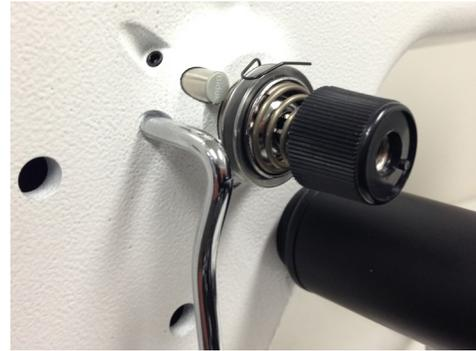
3. Continue to test the stitching on the fabric scrap and adjust by turning the tension dial until you are happy with the stitches.
