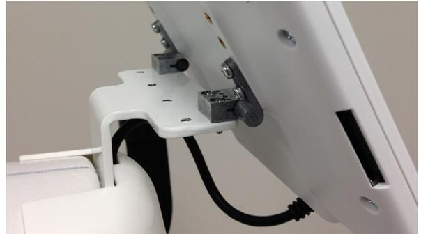
3. Plug the USB mini B cable (with 90° connection), coming out of the top front cover, into the bottom of the display. This cable provides power and signal connection from the machine to the display. The USB connection on the bottom right of the display is used for updating the display and the machine software.
