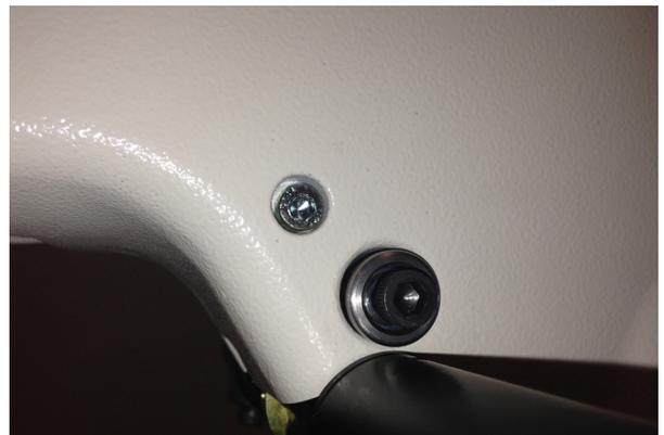
7. Connect the handlebar's USB mini B cables into the side of the machine. Connect the longer cable coming from the handlebar to the bottom connector on the machine and the shorter cable to the closer upper machine connector.
