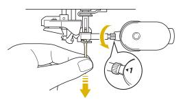
With the flat side of the needle facing the back, insert the new needle all the way to the top of the needle stopper (viewing window) in the needle clamp. Use the multi-purpose screwdriver to securely tighten the needle clamp screw.
