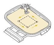
• Do not lower the needle when the embroidery frame is moving. If the needle is down, it could break and result in injury.
