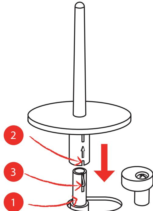
Inserting thread spool
