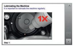
> Give one drop of oil in each of the two oil depots so that the felts are damp and make sure that the redmarked surface of the hook sleeve remains free of oil.
