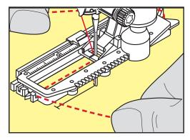
> Pull the cord on the left side under the buttonhole foot to the front with slide.
