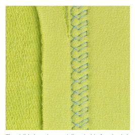
The visible hem is especially suitable for elastic hems in jersey, cotton, wool, synthetic and blended materials.
