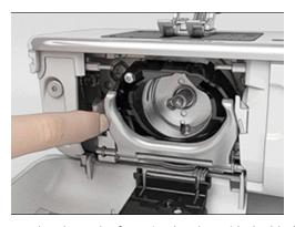
> Flap down the fastening bracket with the black hook race cover.
