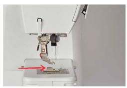
> Lower the shaft via the lever.
