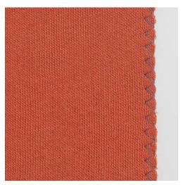
The Zig zag No. 2 is suitable for all materials. It can also be used for elastic seams as well as for decorative sewing. Use darning thread for fine materials. When sewing satin stitch, it is recommended to select a dense, short the zig zag with a stitch length of 0.5 - 0.7 mm. The satin stitch can be used for appliqué and for embroidering.
