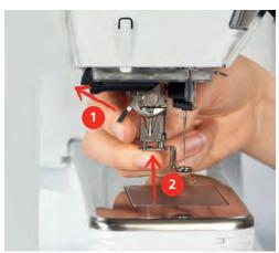
> Press the clamping lever down.
