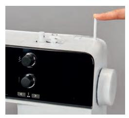
Inserting foam pad and thread spool
