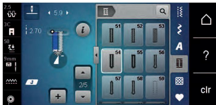
– The machine sews the upper bartack and secures automatically.
