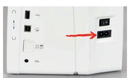
> Insert the plug of the power cable into the electrical outlet.
