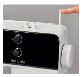
Inserting foam pad and thread spool
