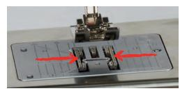
With a short stitch length, the steps are very short. For example when sewing buttonholes and satin stitches. The fabric is fed slowly under the presser foot, even when sewing at maximal speed.
