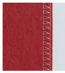
A double overlock seam is suitable for loose knits and cross seams in knits. When working with jersey, a jersey needle should be used to prevent damaging the knit fabric. When sewing stretch materials, use a stretch needle.
