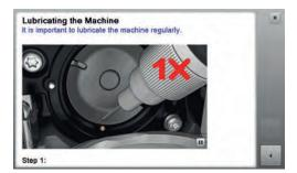
> Give one drop of oil in each of the two oil depots so that the felts are damp and make sure that the redmarked surface of the hook sleeve remains free of oil.
