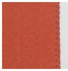
The Zig zag No. 2 is suitable for all materials. It can also be used for eleastic seams as well as for decorative sewing. Use darning thread for fine materials. When sewing satin stitch it is recommended to select a dense, short the zig zag with a stitch length of 0.3 - 0.7 mm. The satin stitch can be used for appliqué and for embroidering.
