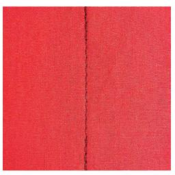
Due to a determined number of 5 stitches sewn forward and 5 stitches sewn backward, the securing is regular.
