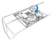
Turn the handwheel to check that the feed dogs move smoothly and do not contact the edges of the slots in the needle plate.
