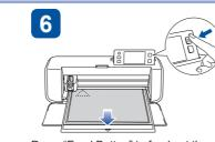
Press "Feed Button" to feed out the mat.
