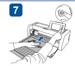
Lightly place your hand on the center of the mat and gently push it forward while pressing the "Feed" button on the operation panel.
