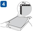
If the adhesive is ok, attach the material onto the mat's adhesive.
