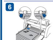
For smooth feeding, align the top of the mat with the guides on the right and left sides of the feed slot and insert it under the feed rollers.
