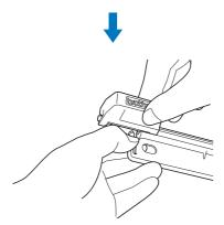
3 Fit the tab on the left side onto the rail of the trimmer.
