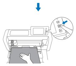
▶ When the material is fed into position, preparation of the roll feeder is completed. At this time, make sure that the left and right feed rollers completely pass over the material.
