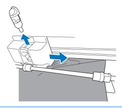
6 Return the feeder release lever (on the right side of the machine) to its original position.
