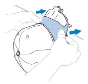
While pulling the lever toward you that is located behind the handle on the right side of the mounting jig, rotate the cap frame to the left. After the cap frame has been rotated 90°, release the lever to lock the cap frame in place.
