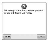
The memory capacity of the USB media has been exceeded.
