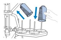
Tie the end of the thread on the new spool with the end of the thread remaining from the previous color.
