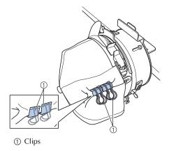
While pulling the lever toward you that is located behind the handle on the right side of the mounting jig, rotate the cap frame to the right.
