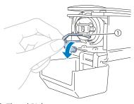
① Thread Picker To gain access to the bobbin case easily, pull the thread picker toward front.
