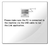
Machine failed to communicate with the PC in the Link mode. Turn off the machine, and on again.
