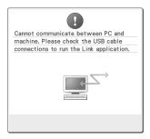
Machine cannot receive any data from the PC in the Link mode. Turn off the machine, and check the USB connection. After connect the USB cord securely, turn on the machine again. (Refer to page 176)
