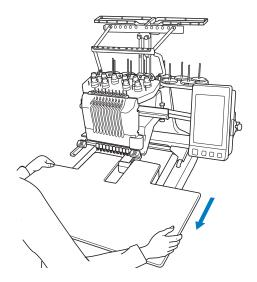
Tighten the thumb screws on the table.
