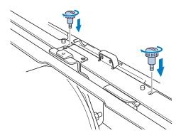
While pushing in the cap frame driver toward the machine so that it is fully inserted, tighten the two lower thumb screws to secure the cap frame driver.
