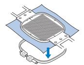
Press the inner frame into the outer frame. Remove the embroidery sheet.
