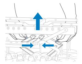
After the thread guide assembly support is extended and the thread guide assembly is raised to its highest position, tighten the two thumb screws to secure the thread guide assembly in place.
