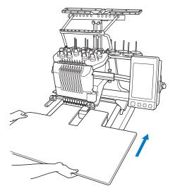
While looking below the table, lightly lift it up, and then lower it so that the screw fits into the notch at the front of the guide plate.
