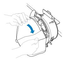
Use the clips to secure the cap.
