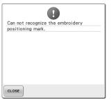
Machine failed to recognize the embroidery positioning mark. Confirm that the embroidery positioning mark is in the selected area. If problem persists, reposition the mark.
