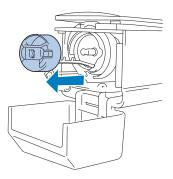
Rotate the handwheel (about 50 degrees) to move the race of the hook to a position where it can easily be oiled.
