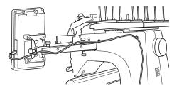
Plug the USB cable connector into the corresponding USB ports for the computer and for the machine.
