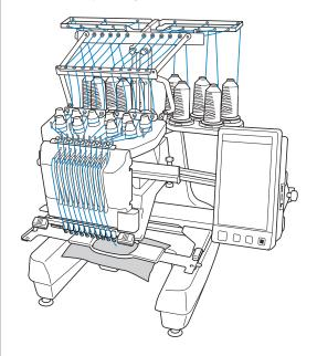
Not all ten needles can be used to sew at the same time. Only one needle is moved to the embroidering position at a time. According to the sewing order, the needle bar case is moved to the left and right so that the needle bar and needle thread with the required color can be moved to the embroidering position.
