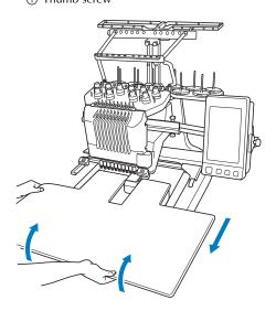
After the pins on each side reach the notches in the guide plates, raise the table to lift the pins up through the notches.
