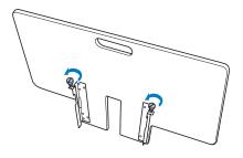
Position the table so that the notch at the center aligns with the machine bed, and then place the table flat on the guide plates.
