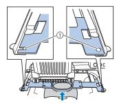
① Make sure that the pins on the left and right arms of the embroidery frame holder fit into the positioning slot and hole on the embroidery frame.
