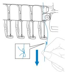
Continue pulling the thread until the knot is above the needle. Cut the knot.
