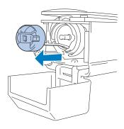
Slide the paper under the tension-adjusting spring to remove any dust.
