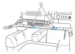
① Use the thumb screws included with the machine (thumb screws removed in step 1) on page 261).
