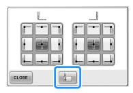
▶ The needle bar is positioned in the lowerleft corner of the pattern. The embroidery frame moves so that the needle is positioned correctly.
