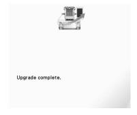
Unplug the USB cable, and turn the machine off and on again.
