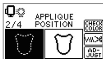
▶ The position for the appliqué is stitched, and the sewing machine stops. "APPLIQUE" will be displayed on the screen.
