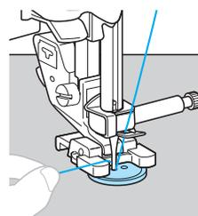
▶ The sewing machine automatically stops after sewing reinforcement stitches.
