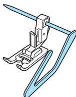
**2** Adjust the stem of the quilting guide so that the guide aligns with the seam that has already been sewn.
