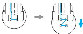
**7** Turn the handwheel toward you (counterclockwise) to check that the needle correctly goes into the two holes of the button. Adjust the stitch width to the distance between the button holes.
