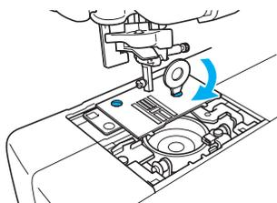
Turn the handwheel to check that the feed dogs move smoothly and do not contact the edges of the slots in the needle plate.
