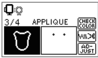
▶ The position for the appliqué is stitched, and the sewing machine stops.
