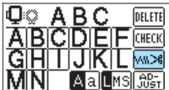
2 Press to turn off the automatic thread cutting ().
