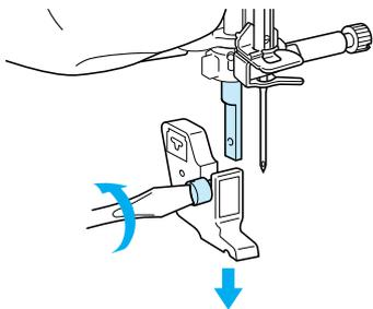
**3** Set the operation lever of the walking foot so that the needle clamp screw is set between the fork, and position the walking foot on the presser foot bar.
