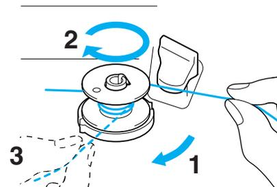
**8** Pass the end of the thread through the guide slit in the bobbin winder seat, and pull the thread to the right to cut the thread with the cutter.
