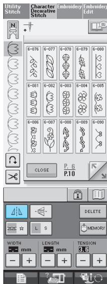
→ The pattern is flipped along a vertical axis.
