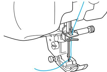
→ The upper threading is finished.
