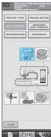
→ The screen shows instructions for threading the machine.
