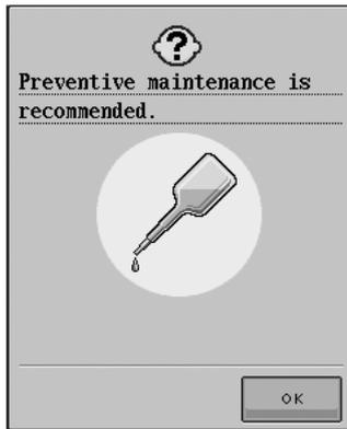
Once this message appears, it is recommended to take your machine to an authorized retailer for a regular maintenance check. Although this message will disappear and the machine will continue to function once you press **OK**, the message will display several more times until the appropriate maintenance is performed.
