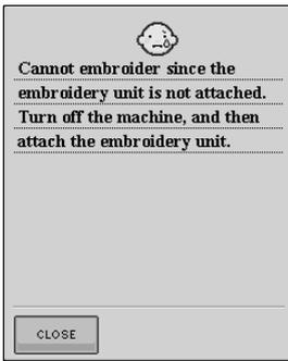
This message is displayed when the "Start/Stop" button is pushed and the machine is in embroidery mode, but the embroidery unit is not attached.
