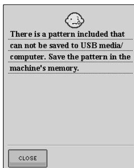
This message is displayed when you try to save a copyright protected pattern to USB media/ Computer. According to copyright laws, patterns that are illegal to reproduce or edit cannot be saved to floppy disks. If this message displays, save the pattern in the machine's memory.
