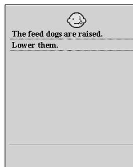
This message is displayed when the "Start/Stop" button is pushed without raising the feed dogs after the feed dogs are lowered or after the embroidery unit is attached.
