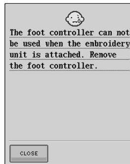
This message is displayed when the foot controller is pressed while the embroidery unit is attached.
