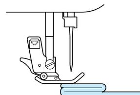
→ The presser foot remains level, enabling the fabric to be fed.
