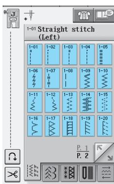
→ The symbol of the correct presser foot will be displayed in the upper left corner of the LCD.
