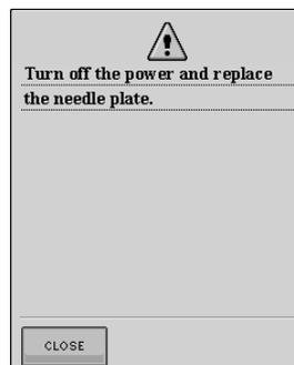
This message is displayed when you try to sew with a stitch other than a middle needle position while the single-hole needle plate is installed. This message is displayed when the needle plate is removed with the machine on or when the machine is turned on in the embroidery or embroidery edit mode.
