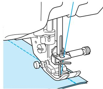
**7** After sewing, press the "Thread Cutter" button to trim the threads.
