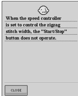
This message is displayed when the speed control lever is set to control the zigzag stitch width, and the "Start/ Stop" button is pushed. Use the foot controller to operate the machine.
