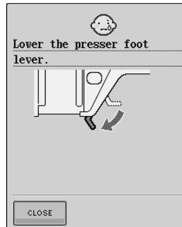
This message is displayed when the "Presser Foot Lifter" button is pushed while the presser foot lever is raised/the needle is lowered.
