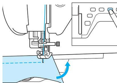
When edge stitching a short stitch length close to the edge of the fabric, the presser foot may not cover enough fabric for proper feeding. Before you begin to sew, sew a basting thread at the corner point. When you change direction at the corner, start sewing as you pull the basting thread toward the back.
