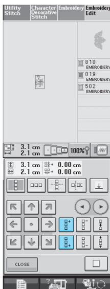
**5** Adjust the spacing of the repeated pattern.
