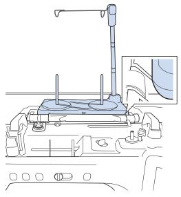
Place the spool of thread on the spool pin so that the thread feeds off the spool clockwise. Firmly insert the spool cap onto the spool pin.
