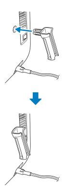
With the flat part of the dual purpose stylus facing to the machine, insert it into the dual purpose stylus holder.
