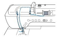
Pass the thread through the needle bar thread guides on the needle bar, then thread the needle on the left side manually.
