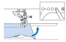
The pivot setting is useful when changing the sewing direction. When the machine is stopped at the corner of the fabric, the machine stops with the needle in the fabric and the presser foot is automatically raised so the fabric can easily be rotated ("Pivoting" on page 89).
