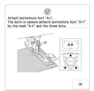
This message appears when start sewing buttonhole stitches without attaching buttonhole foot "A+".
