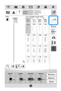
→ The key appears as ເດ , the quilting foot is raised to the necessary height, and then the feed dogs are lowered for free motion sewing.
