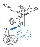
6 Tighten the screw with the included screwdriver (large).
