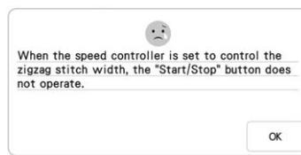
This message is displayed when the speed control lever is set to control the zigzag stitch width, and the “Start/ Stop” button is pushed. Use the foot controller to operate the machine.
