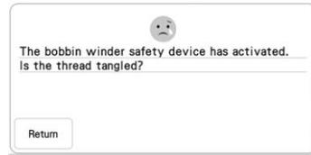
This message is displayed when the bobbin is being wound, and the motor locks because the thread is tangled, etc.
