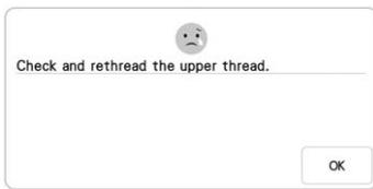
This message is displayed when the upper thread is broken or not threaded correctly, and the "Start/Stop" button or the "Reverse/ Reinforcement Stitch" button is pressed.
