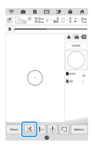
Press **\*** to turn off the thread trimming function.
