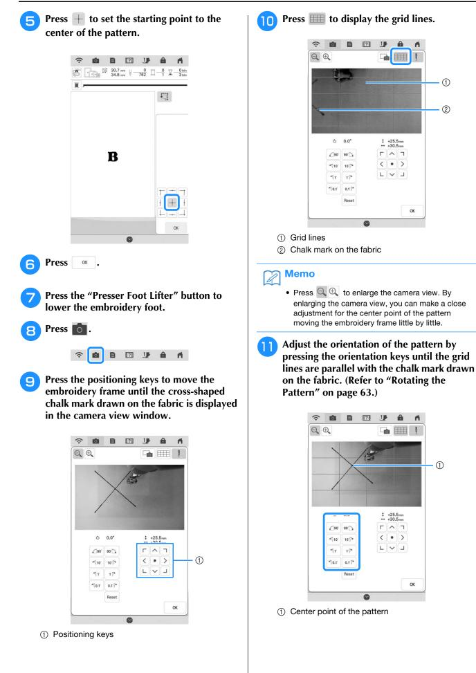
Press the positioning keys to move the embroidery frame until the center point of the pattern in the camera view window is aligned with the chalk mark drawn on the fabric.
