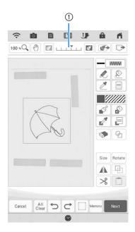
\* After the scanned image is converted to stitching, it appears as a background in the pattern drawing screen. Use gauge ① to adjust the transparency of the background. Each press of 🔝 lightens the
