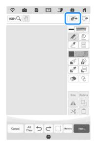
Press , press shape registered in step , and then arrange it over the scanned pattern.
