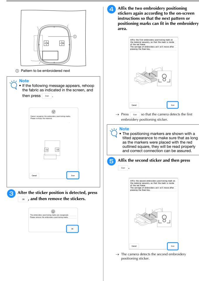
After the two embroidery positioning stickers have been detected, the following message appears. While making sure that the embroidery positioning stickers do not peel off, rehoop the fabric according to the example displayed on the on-screen instruction.
