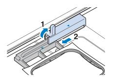
Insert a wound bobbin into the machine. (Refer to "Setting the Bobbin" on page 20.)
