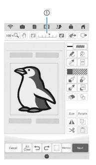
\* After the scanned image is converted to stitching, it appears as a background in the pattern drawing screen. Use gauge 1 to adjust the transparency of
