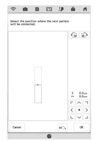
You can adjust the position of the second pattern using the keys described below.
