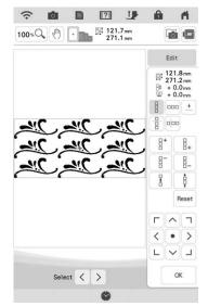
• When changing the direction in which the pattern will be repeated, all of the patterns in the red frame will automatically be grouped as one repeating unit. Refer to the following section on how to repeat one element of a repeated pattern.
