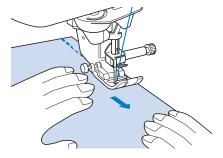
4 End the basting with reinforcement stitches.
