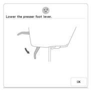
This message is displayed when the "Presser Foot Lifter" button is pushed while the presser foot lever is raised/the needle is lowered.
