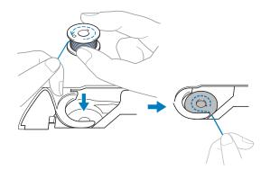
Lightly hold down the bobbin with your right hand (①), and then guide the end of the thread around the tab of the needle plate cover with your left hand (②).
