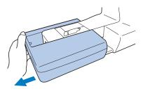
**3** Slide the tab on the cover of the connection port in the direction of the arrow to open the cover.
