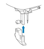
Hold the presser foot holder in place with your right hand, and then tighten the screw using the screwdriver in your left hand.
