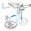
Tighten the screw with the included screwdriver. 5
