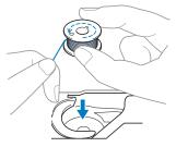
If the bobbin is inserted with the thread unwinding in the wrong direction, sewing will be done with an incorrect thread tension.
