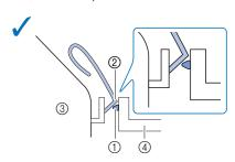
Notch (1) does not fit firmly under the bend in the lever (2).
