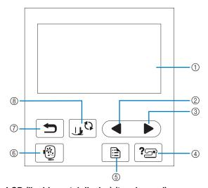
LCD (liquid crystal display) (touch panel) Selected pattern settings and messages are displayed.
