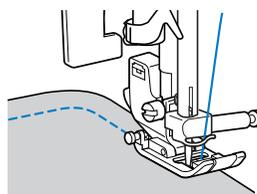
When sewing along a curve while using a zigzag stitch, select a shorter stitch length in order to obtain a finer stitch.
