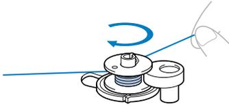
**11** Pass the end of the thread through the slit in the bobbin winder seat, and then pull the thread to the right to cut it.
