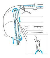
Pass the thread behind the needle bar thread guide.
