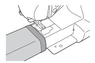
When you are finished with free-arm sewing, install the flat bed attachment back in its original position.
