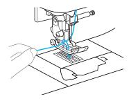
Pull out about 10 cm (4 inches) of the bobbin thread under the presser foot toward the rear of the machine.
