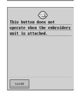
This message is displayed when the "Reverse/Reinforcement Stitch" button is pushed while the embroidery unit is attached.
