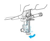
Use the included screwdriver to firmly tighten the screw of the presser foot holder.
