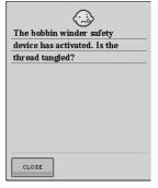
This message is displayed when the bobbin is being wound, and the motor locks because the thread is tangled, etc.
