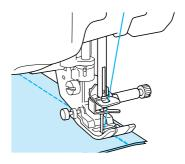
After sewing, press the "Thread Cutter" button to trim the threads.
