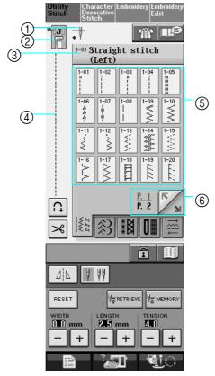
① Shows single or twin needle mode setting, and the needle stop position.
