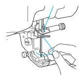
Pass the thread through the presser foot, and then pull out about 100-150 mm (approx. 4-6 inches) of thread toward the back of the machine.
