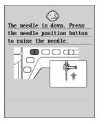
This message is displayed when the embroidery unit is attached and the power is turned on with the needle in the down position.
