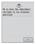
This message is displayed when replacing the embroidering bobbin thread.
