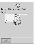
This message is displayed when the "Presser Foot Lifter" button is pushed while the presser foot lever is raised/the needle is
