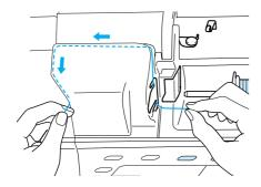
When finished pulling the thread through the thread guide, cut the thread and leave the thread in position.
