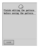
This message is displayed when the "Start/ Stop" button is pushed while the machine is in embroidery edit mode and a pattern is being edited.
