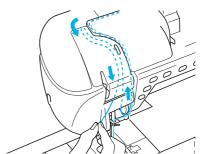
Do not pass the thread in the needle bar thread guides on the needle bar. Thread the needle on the right side.
