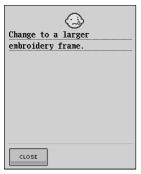
This message is displayed when the machine is in embroidery mode and the small frame is attached, and the selected pattern does not fit in the small frame.
