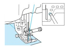
Press the "Thread Cutter" button to trim the threads.
