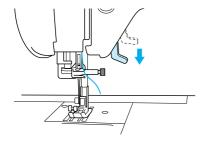
Holding the thread with both hands, pass the thread through both the upper and lower needle bar thread guides.
