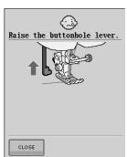
This message is displayed when the buttonhole lever is down, a stitch other than a buttonhole is selected, and the "Start/ Stop" button or the "Reverse/ Reinforcement Stitch" button is pushed.
