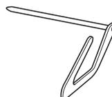
① **Insert the stem of the quilting guide into the hole at the rear of the walking foot or presser foot holder.**
