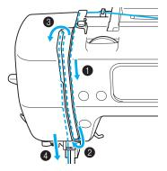
Make sure that the thread is passed into the thread take-up lever as shown below.
