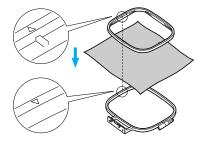
Tighten the adjustment screw by hand just enough to secure the fabric.
