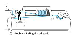
Slide the bobbin winder shaft to the left, and then remove the bobbin from the shaft.
