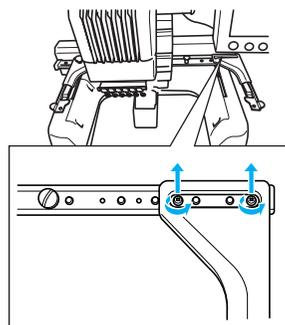
**5** Remove the right arm, align the pins on the embroidery frame holder with the holes in the arm, as shown in the illustration, and then insert the screws removed in step 4 and tighten them.
