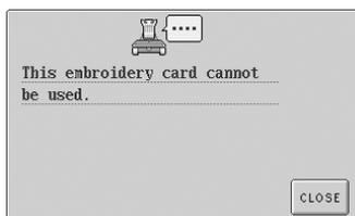
**A pattern on an embroidery card not compatible with this machine was being recalled.**
