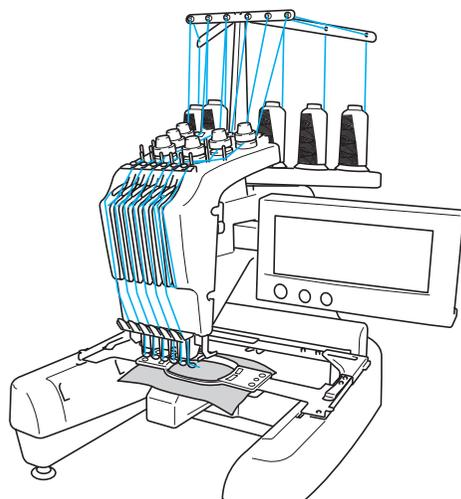
Not all six needles can be used to sew at the same time. Only one needle is moved to the embroidering position at a time. According to the sewing order, the needle bar case is moved to the left and right so that the needle bar and needle thread with the required color can be moved to the embroidering position.
