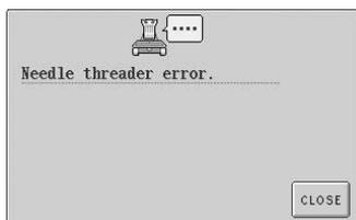
**The automatic needle-threading mechanism did not operate correctly.**
