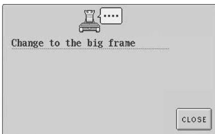
The embroidery machine detects which embroidery frame is installed according to the position of the left arm of the embroidery frame holder. Therefore, the embroidery frame size is determined by the position of the left arm, even if the detected embroidery frame is not actually installed. In addition, if the embroidery frame holder is not installed, the embroidery machine determines that the cap frame (sold separately) is installed.
