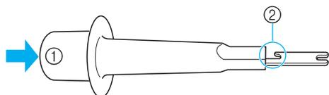
**4** While holding the needle in place with your left hand, tighten the needle set screw.
