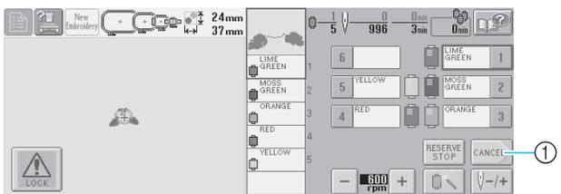
In the **embroidering screen**, check the thread colors assigned to the needle bars, and then install
