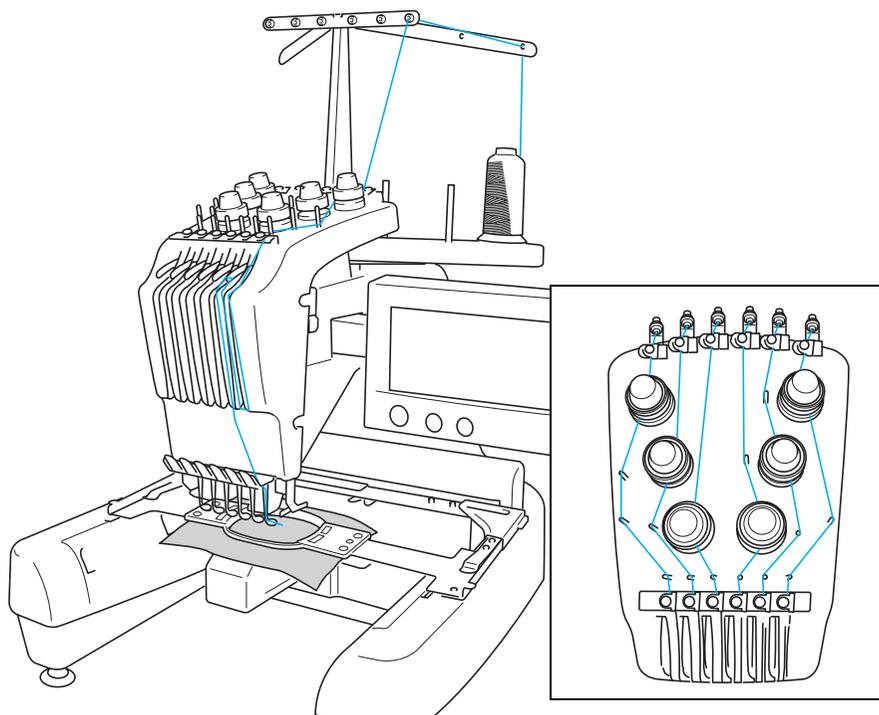
The numbers indicate the thread path for each of the numbered needle bars. Be very careful to correctly thread the needle bars.
