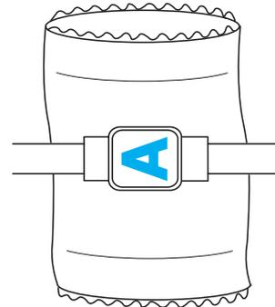
Example: When embroidering a T-shirt Rotate the pattern 180 degrees. Pass the machine bed through from the waist of the T-shirt, not from the neck, and attach the embroidery frame to the machine. Prevent the neck to be stretched when the embroidery frame is moved.
