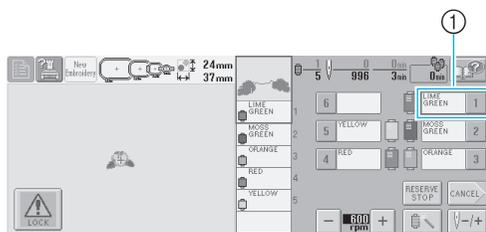
① A red frame around the thread information box indicates which needle bar is currently being used for sewing.
