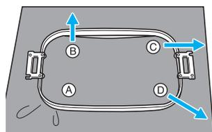
First, align the inner and outer frames at the corner with the screw **A**. Then, while lightly pulling the fabric in the direction indicated by arrow **B** so that the fabric is taut, insert the inner frame at corner **B**. In the same way, lightly pull the fabric in the direction indicated by arrow **C** and insert corner **C**, and then
