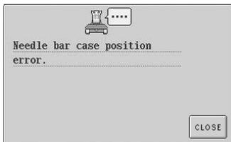
**The needle bar case has stopped at an incorrect position.**
