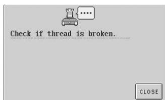
**The upper thread was cut or the thread came out the thread tension disc or a thread guide. The machine is not threaded correctly.**
