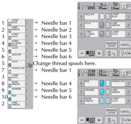
Since the thread colors on needle bars 2 and 3 will be used again after the thread spools are changed, they will not be replaced. However, different colors are assigned to the other needle bars.
