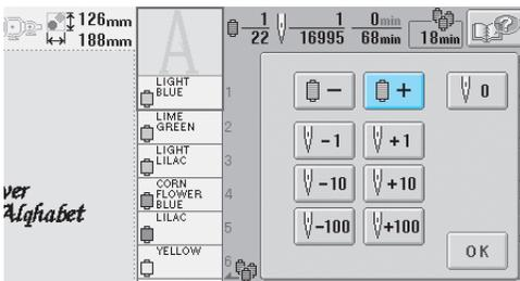
► Each time this key is touched, the next color in the thread color sequence display is selected. After reaching the last color in the thread color sequence display, the scrolling stops.
