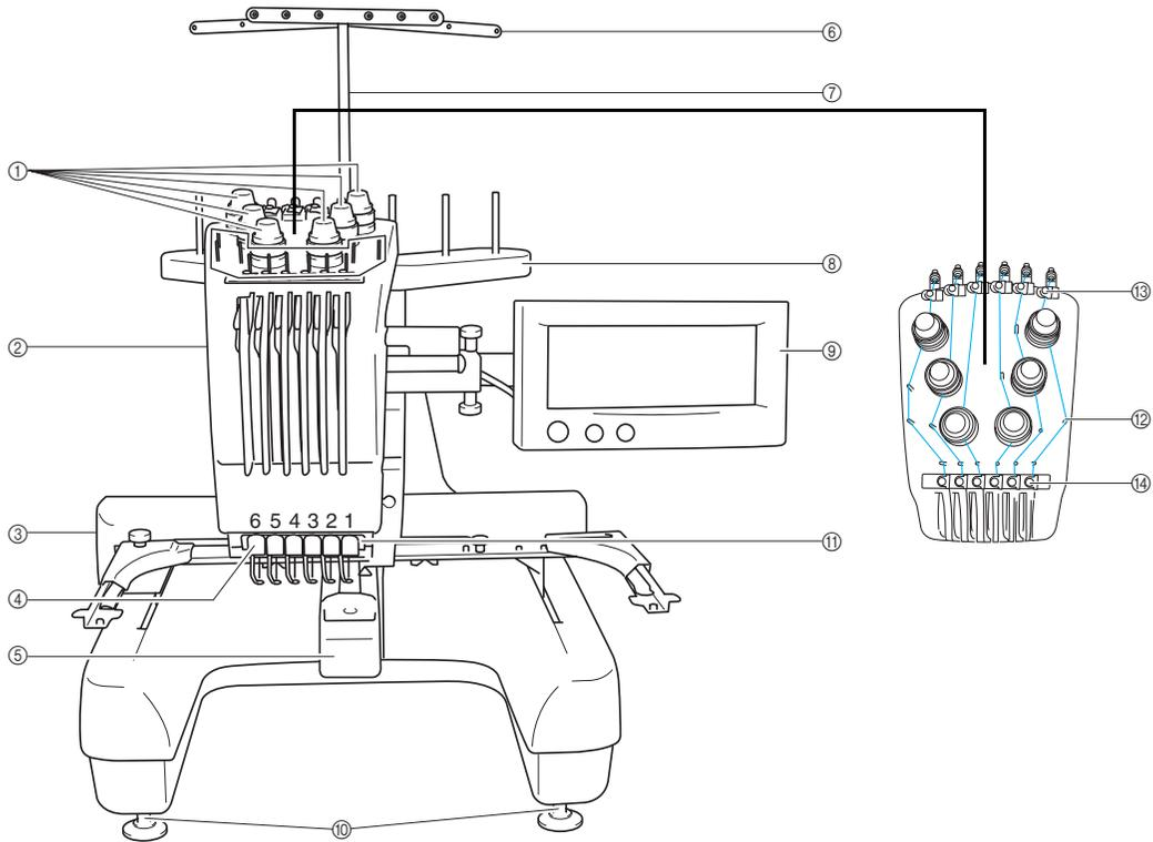
① **Thread tension knobs**
