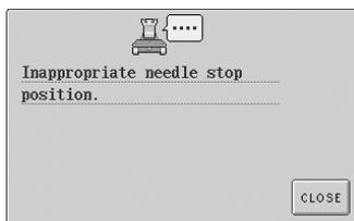
**The needle has stopped at an incorrect position.**
