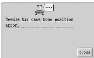
**The needle bar case cannot be moved to its initial position.**
