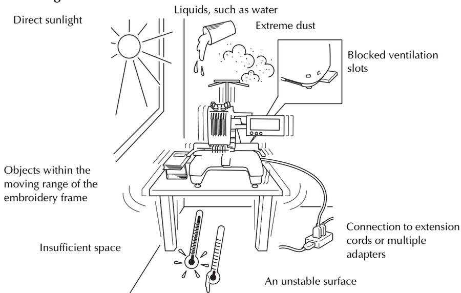
Extremely high or extremely low temperatures (The operating environment should be between 5 °C (40 °F) and 40 °C (104°F))
