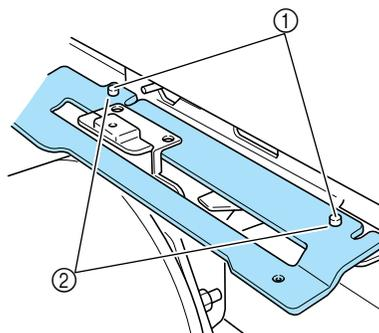
① Pins on the frame-mounting plate of the carriage
