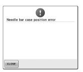
The needle bar case has stopped at The needle bar case motor has locked up. an incorrect position.
