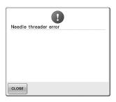
The automatic needle-threading mechanism did not operate correctly.
