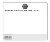
Touch CLOSE to automatically reset the needle bar case.
