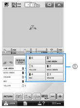
① The threads threaded on the needle bars are indicated as shown here.
