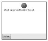
The upper thread broke, the thread came out of the thread tension disc or a thread guide, or the machine is not threaded correctly.
