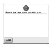
The needle bar case could not be moved to its initial position.
