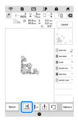
Press to turn off the automatic thread cutting function.
