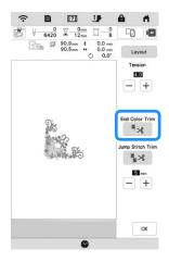
→ The key will display as \_\_\_\_\_\*. When one color thread is embroidered, the machine will stop without cutting the thread.
