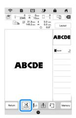
6 Press to turn off the thread cutting function and then press K.
