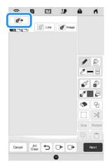
Press , press to recall the stamp shape registered in step 3, and then arrange it over the loaded pattern.
