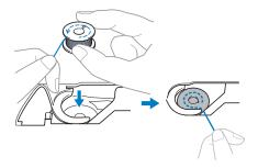
Lightly hold down the bobbin with your right hand (1), and then guide the end of the thread around the tab of the needle plate cover with your left hand (2).
