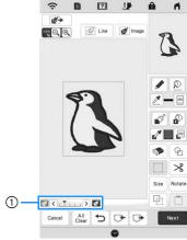
\* After the loaded image is converted to stitching, it appears as a background in the pattern drawing screen. Use gauge ① to adjust the transparency of the background. Each press of lightens the background, making the illustration pattern darker. Each press of darkens the background, making the illustration pattern lighter.
