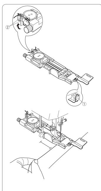
Place the button on the button holder on the buttonhole foot.
