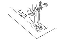
9 Press the start/stop button. The machine will sew "R&B", cut the threads and stop automatically.
