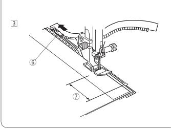
2 Attach the zipper foot E. Adjust the stitch width to 7.5–8.5.
