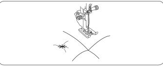
You can close quilt layers by using the clasp stitch. Select stitch pattern 06 (mode 2). Press the memory key. Select locking stitch (pattern 87 (mode 2)). Start sewing.
