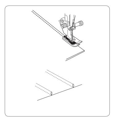
Fold the fabric with the wrong sides together. Place the folded fabric under the blind hem foot.
