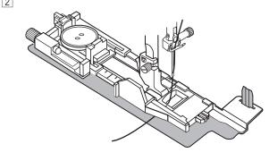
3 Place the fabric between the buttonhole foot and stabilizer plate. Lower the needle into the starting point by turning the hand wheel.
