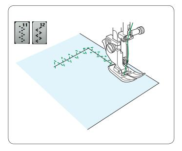
**U11, U12 Multiple zigzag stitches** These stitches are used for mending tears.
