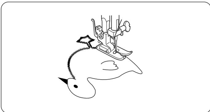
Baste (or fuse with iron-on fabric joiner) applique pieces on the fabric. Stitch around the applique making sure the needle falls along the outer edge of the applique. When sewing corners, lower the needle down into the fabric. Raise the presser foot and pivot the fabric to the right or left.
