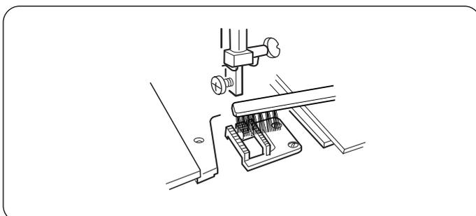
Remove the needle and the presser foot.
