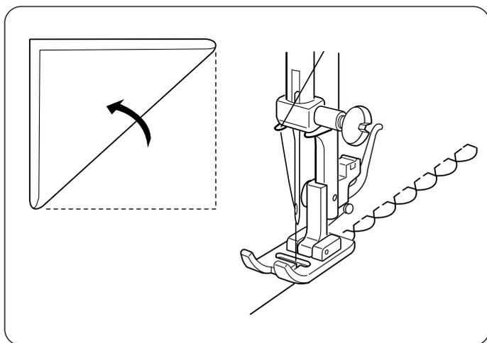
Place the folded edge along the slot of foot.
