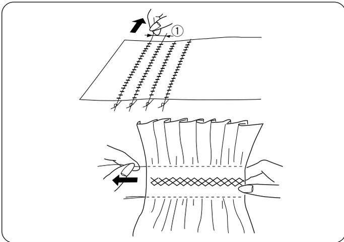
With the stitch length at "4", sew straight stitching lines 1 cm (3/8") apart, across the area to be smocked. Knot the threads along one edge. Pull the bobbin threads and distribute the gathers evenly. Secure the threads at the other end. Sew the decorative stitch between the gathering stitches. Pull out the gathering stitches.
