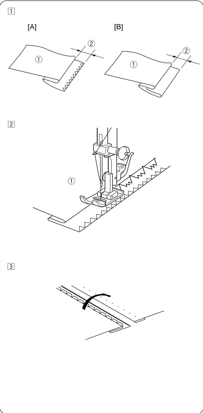
① On heavyweight fabrics that ravel, the raw edge should be overcast first. Then fold the hem, as illustrated, leaving 1/4" (0.7 cm) of the hem edge showing.
