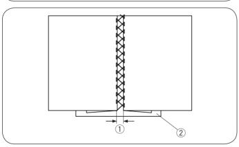
Use this stitch to join two pieces of fabric to create an open work appearance and add design interest. Fold under each fabric edge 5/8" (1.5 cm) and press. Pin the two edges to paper or tear away backing 1/8" (0.3 to 0.4 cm) apart. Sew slowly, guiding the fabric so the needle catches the folded edge on each side.
