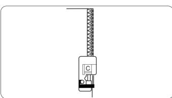
This stitch can be used for sewing fabrics that tend to fray extensively such as linens and gabardines.
