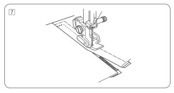
Open the zipper, then lower the foot and stitch the remainder of the seam. After finished sewing, remove the basting stitches on the upper fabric.
