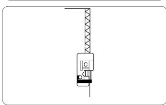
This stitch is used to simultaneously seam and overcast edges of fabrics. Use this stitch when you do not need to open seams flat.
