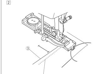
2 Start the machine and sew the buttonhole. Each side of the buttonhole and the bartacks will be sewn over the cord.
